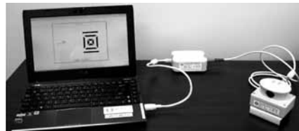
Electrical impedance myography. A portable device (Skulpt Inc., Boston, Mass.) with a simple, handheld wand is used to measure impedance over selected muscles.
